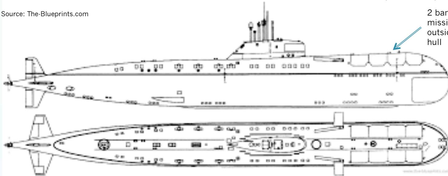
2 banks of 4 cruise missile launchers outside the pressure hull
