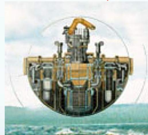
The above diagrams from the Gidropress website likely shows a cross-section of the BM-40A reactor within the outline of an Alfa submarine hull.
