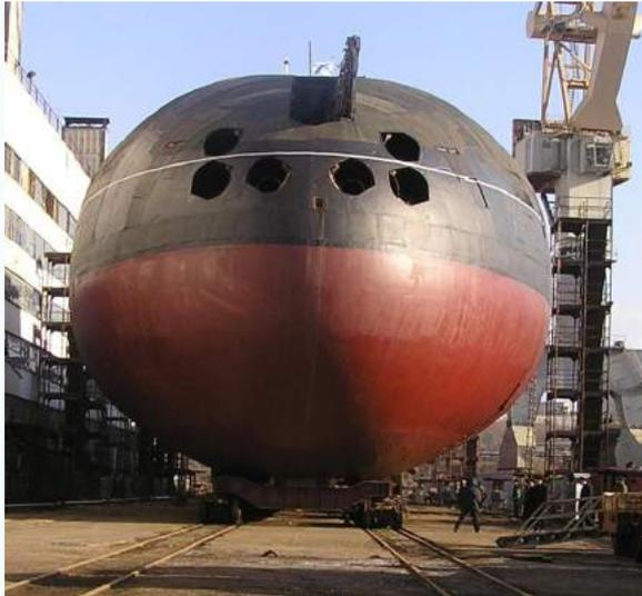
Oscar II-class SSGN with bow torpedo loading hatch & torpedo tube doors open.
