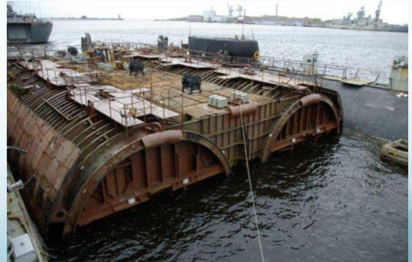
Typhoon reactor compartments afloat.
