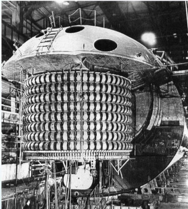
Typical Russian cylindrical bow sonar array, torpedo tubes above
