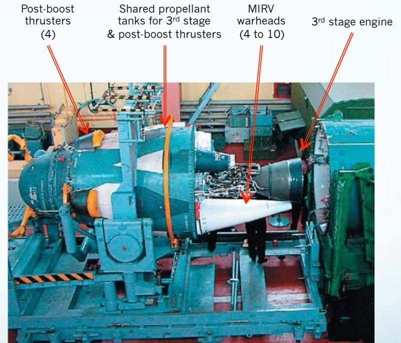
R-29RM 3rd stage and warhead section with some MIRV warheads removed, showing 3rd stage engine installation.
