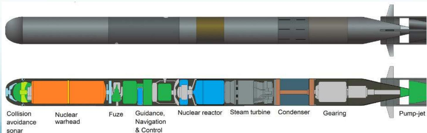
Poseidon / Status-6 /Kanyon torpedo notional cross-section. Source: <http://www.hisutton.com/>
