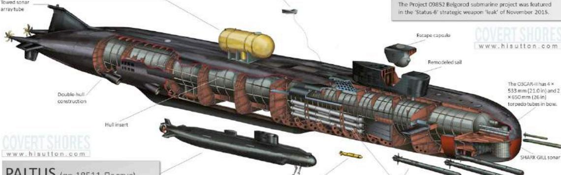
Labels in diagram: Towed sonar array tube, Communication buoy, Escape capsule, Remodeled sail, Double-hull construction, Hull insert, SHARK GILL sonar.
