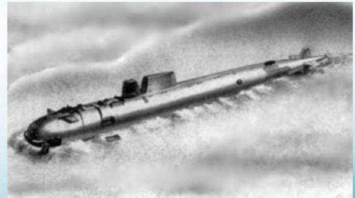
Artist concept of K-278 site. Note cracked hull & missing escape capsule (V-notch) in the sail
