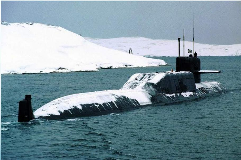
Delta I. Note the distinctive notch at the back of the missile deck.
