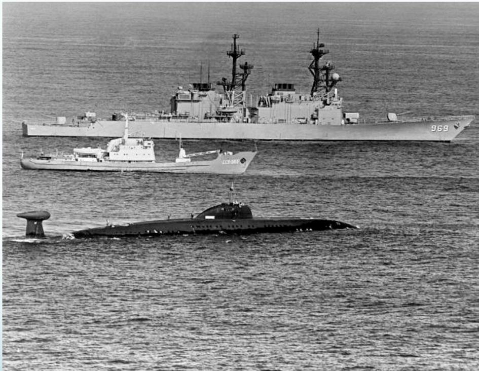
Victor III K-324 on the surface in October 1983 with a Moma class survey vessel and US Spruance-class destroyer USS Peterson (DD-969) after K-324 damaged its propeller on the towed array sonar of another US Navy ship near Bermuda.
