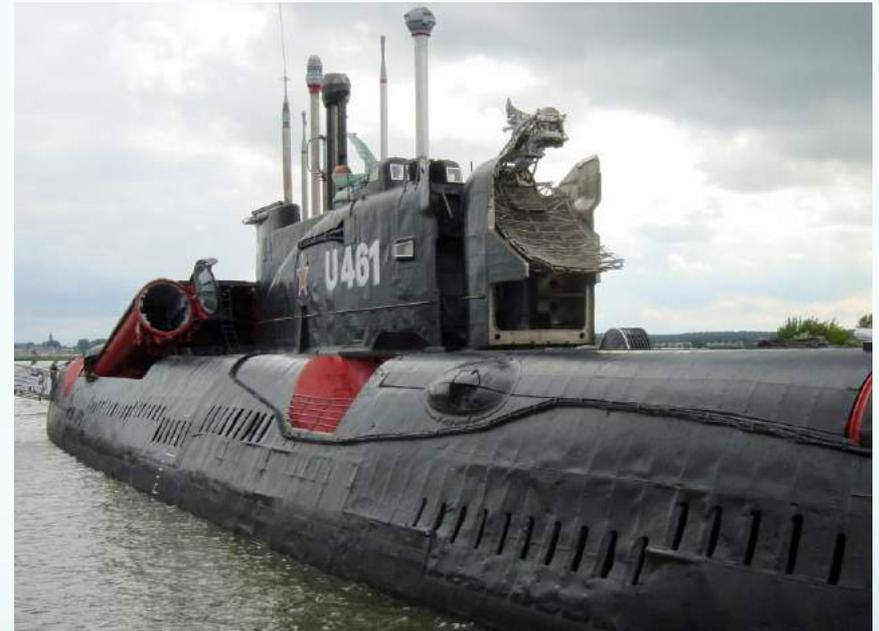
Above: Large guidance antenna for anti-ship cruise missile mid-course guidance was built into the forward edge of the sail structure, which opened by rotating.
