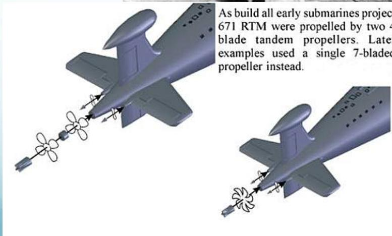
As build all early submarines project 671 RTM were propelled by two 4 blade tandem propellers. Later examples used a single 7-bladed propeller instead.
