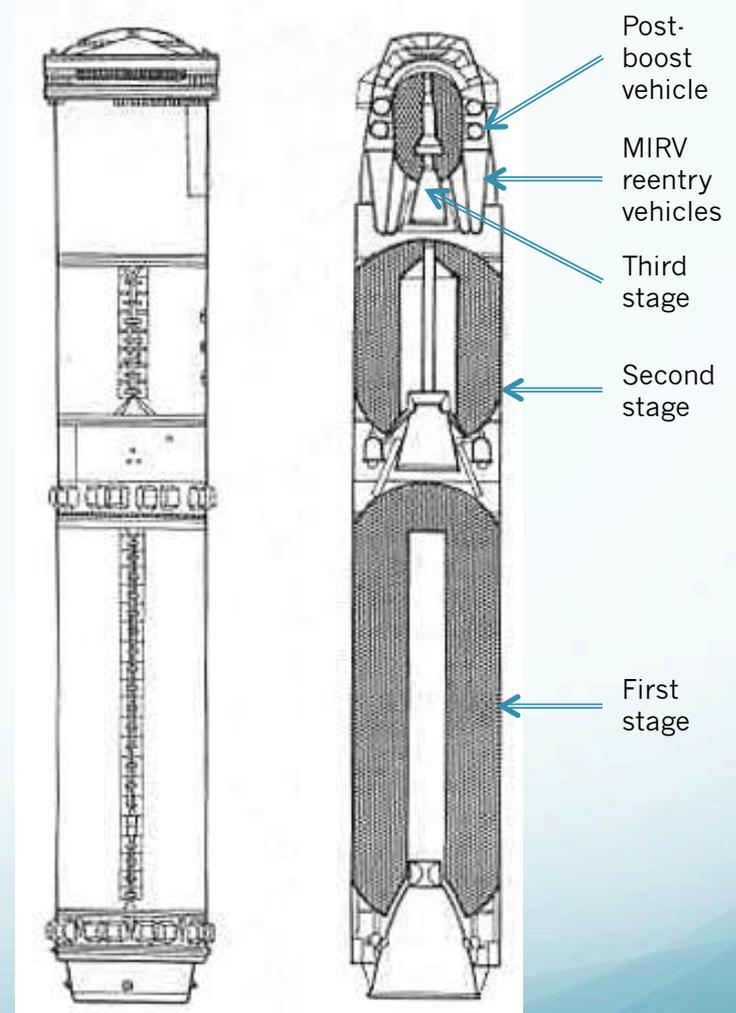
R-39 missile storage canister (left) and missile cross-section (right). Source: adapted from <http://cakra401.blogspot.com/>
