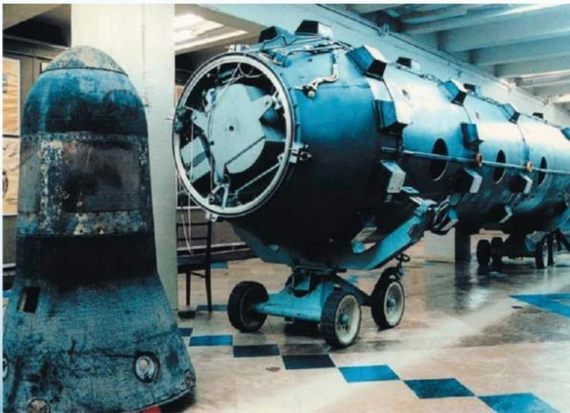
R-27 reentry vehicle (left) and missile casing (right)
