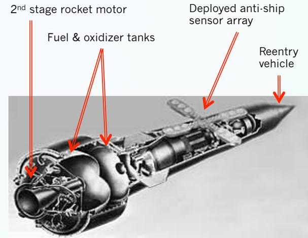
R-27K second stage with anti-ship sensor array deployed.
