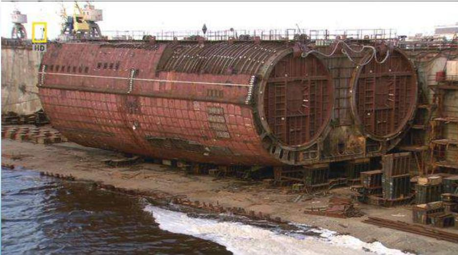
Typhoon reactor compartment removed and sealed.
