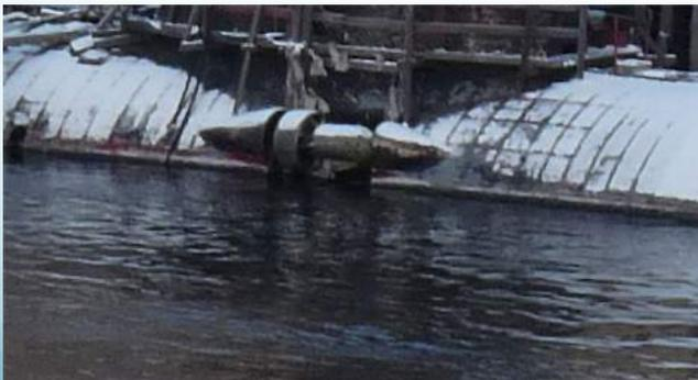
AS-13 right front thruster in retracted position without cover. Source: <http://forums.airbase.ru/>
