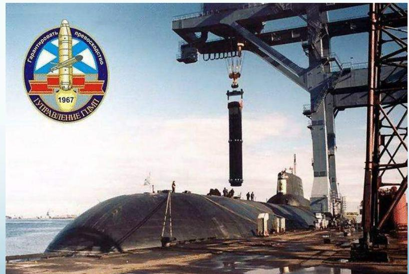
R-39 canister being loaded onto a Project 941 Typhoon-class SSBN.
