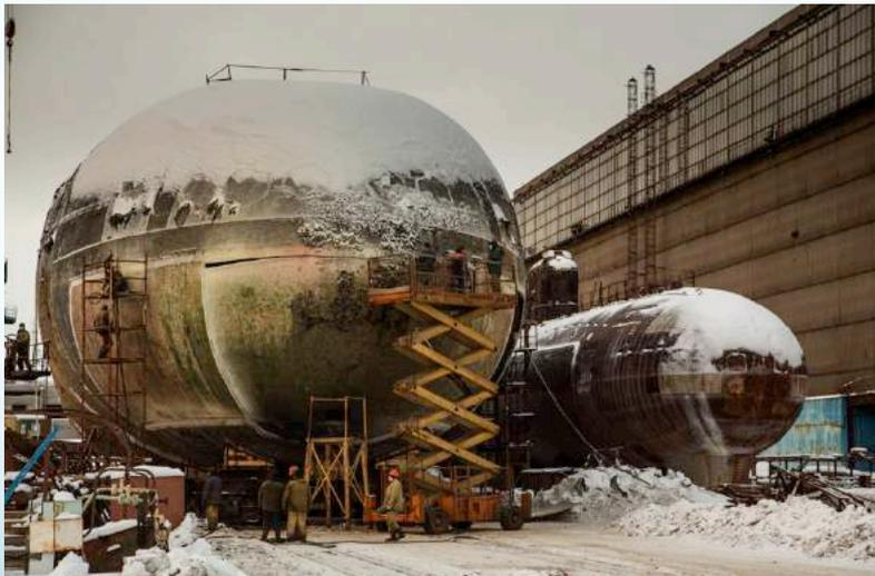
K-3 *Leninsky Komsomol* in drydock at the Nerpa shipyard with the much larger Oscar II K-148 *Krasnodar*, lead ship for the Oscar II class of SSGNs, which was being scrapped (circa 2012 - 2014). Source: <https://www.reddit.com>
