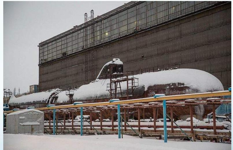
K-3 after cuts in the hull were made to remove the reactor compartment. Source: <http://www.subsim.com/radioroom/>
