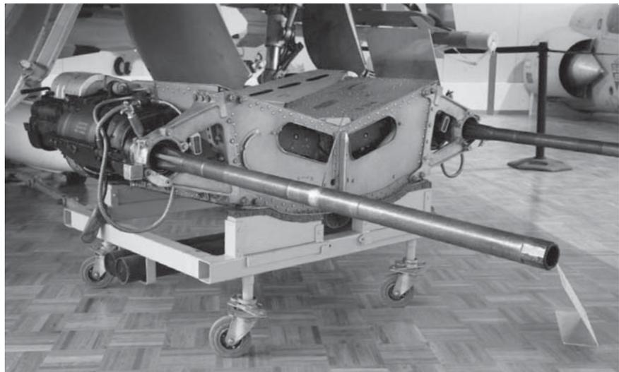
The Mirage IIICJ's only truly effective weapons during the Six Day War were its twin DEFA 552 30mm cannon, neatly housed in a ventral pack that could be lowered out of the jet for servicing and rearming.
