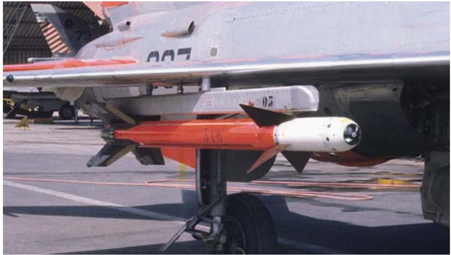
higher than 30,000ft over land or 10,000ft over sea, and a rear hemisphere launch only against a target flying at a lower altitude. R 530 engagement range was one to ten miles, but radar lock had to be achieved prior to launch, and this proved difficult in a combat situation with the unsophisticated Cyrano system fitted in the Mirage IIICJ.
