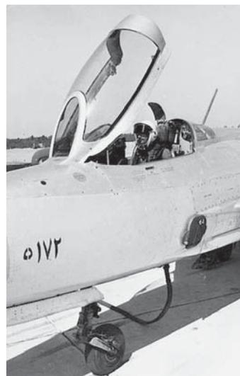
An EAF pilot completes the pre-flight checks of his MiG-21F-13 in 1965. Note that its Arabic serial number, 5172, has been applied with stencils. This seems to have been characteristic of some of the early MiG-21s supplied to Egypt, and might indicate application prior to delivery from the USSR.
