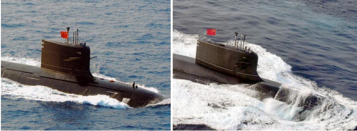
Figure 4. Type 093 with sail modifications (left) and Type 093A sail (right).
